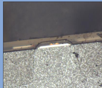
320 \mu\text{m} X 266 \mu\text{m} view of hard disk head slider.
