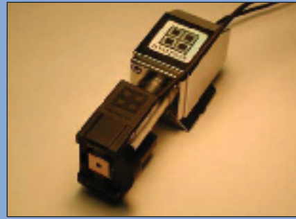
Hysitron's patented three plate capacitive transducer on the TriboScanner™ .
