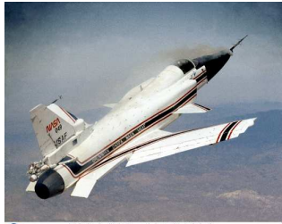
NASA Dryden Flight Research Center Photo Collection http://www.dfc.nasa.gov/gallery/photo/index.html NASA Photo: EC21-611-15 Date: September 13, 1991 X-29 at High Angle of Attack
